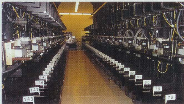
BRAKE LINES: A train’s worth of electronically controlled brakes ganged together for testing. PHOTO: ROBB MANDELBAUM
